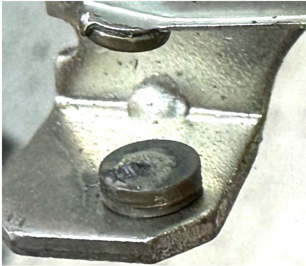
Fig. 6. Marelli severe wear
