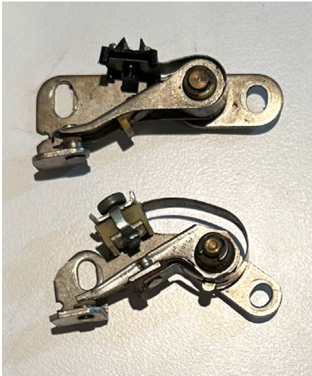
Fig.2. Top, straight points; bottom, curved points
