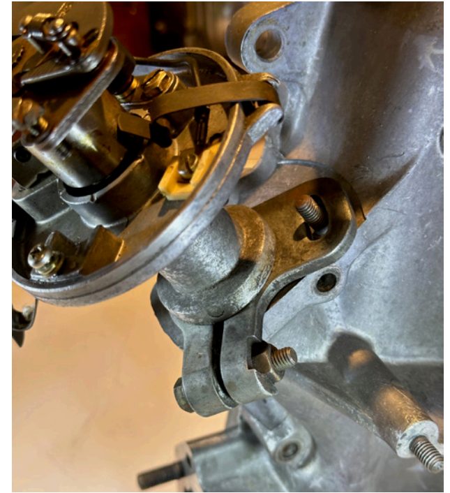
Fig. 6. Suggested orientation of distributor pinch clamp
