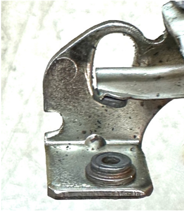
Fig. 11. Standard Motor Products ventilated fixed contact
