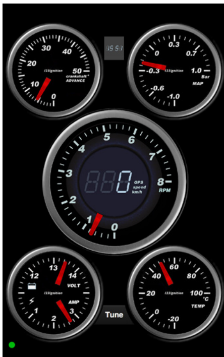
Fig. 7. 123 Tune phone app display of hot idle
