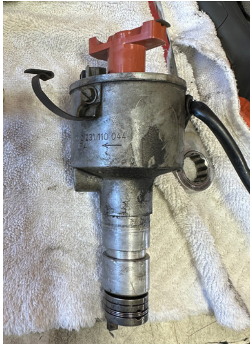
Fig. 3. Earlier type Bosch distributor
