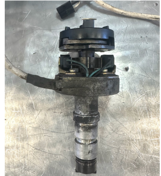
Fig. 4. MarelliPlex distributor with two magnetic pickups
