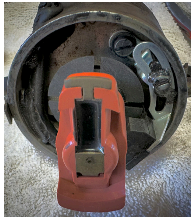
Fig. 8. Earlier Bosch distributor with Crane optical module
