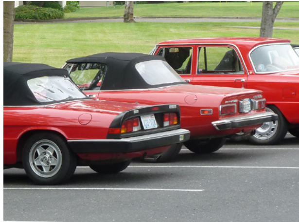
A series 3 tail ( left ) next to a series 2 ( right )
